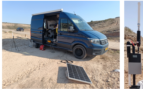
(a) CRAFTER in operation during the field test, with (b) WiFi Bullet access point and solar panel deployed. extender.
