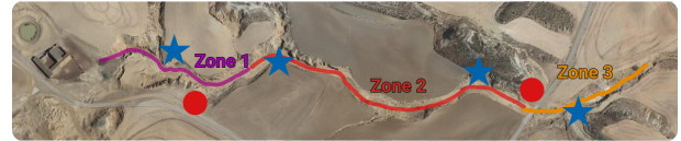
Figure 5: The traversed area is highlighted in this satellite overview. Red circles indicate the two base control station positions and blue stars are the locations of the WiFi extenders at different times during the field trip. The underlying image is taken from Google Maps.
